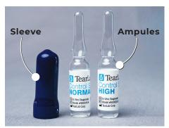
Control Solutions confirm that the Test Cards are working correctly. The glass bottles (ampules) should be kept at room temperature. Do NOT refrigerate or keep in a hot place.
