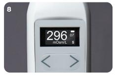
To view previous test results, press either the right (>) or left (<) buttons on the Pen.
